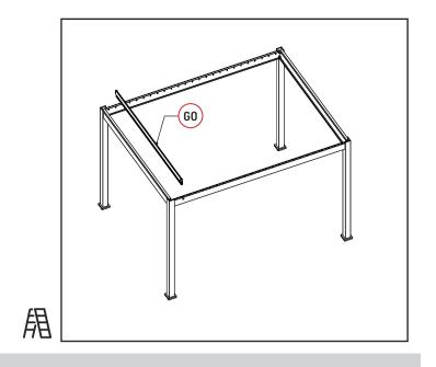
Fasten rubber plugs on both ends of the louvers
