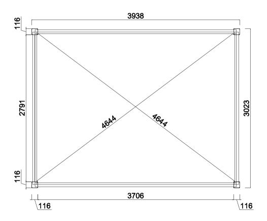
3D FOOTING MEASUREMENT (dimensions in mm)
